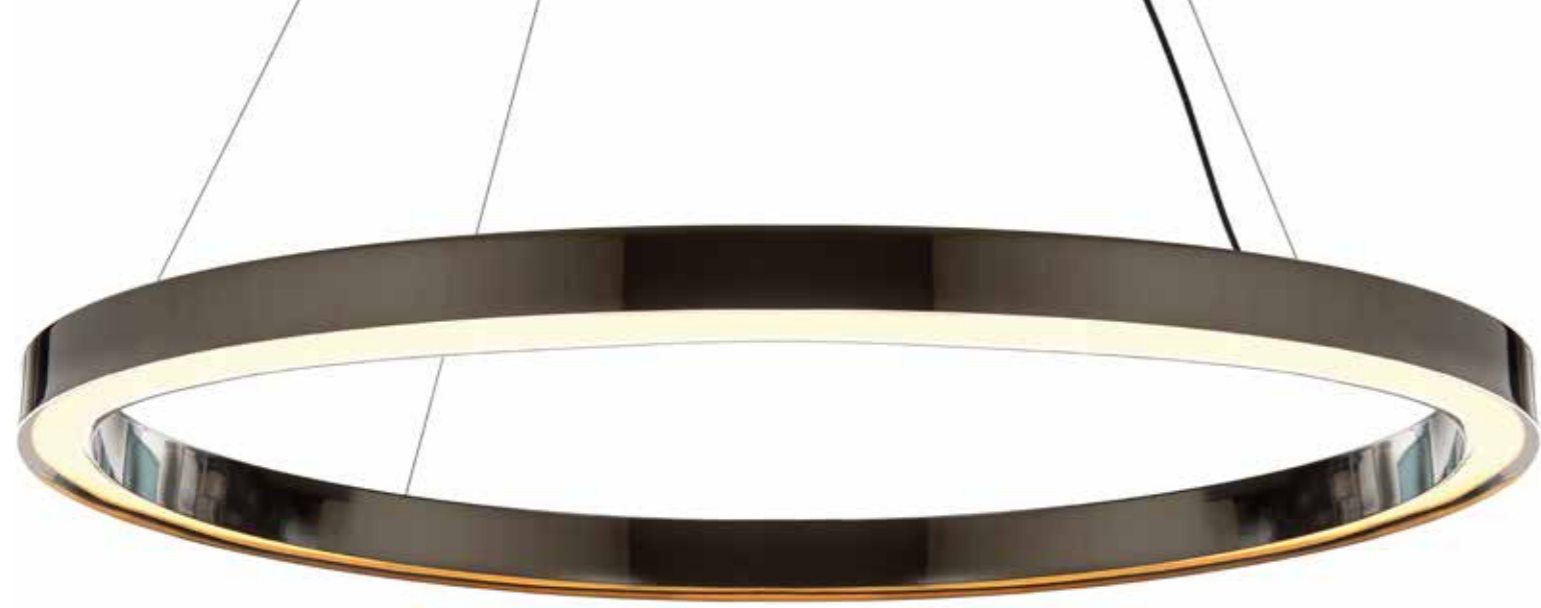
Art. 2103/G/NN/bis Ø 96 cm H 5 cm + 100 cm steel cable Strip Led 3200 K Lumen 5793 85W (Kg 18)
